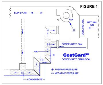
During both heating and cooling operations, the air seal is formed as follows:
